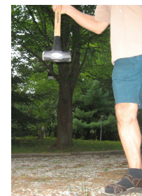
Figure 20: 5 kg sledge hammer drops from 1 meter height.
