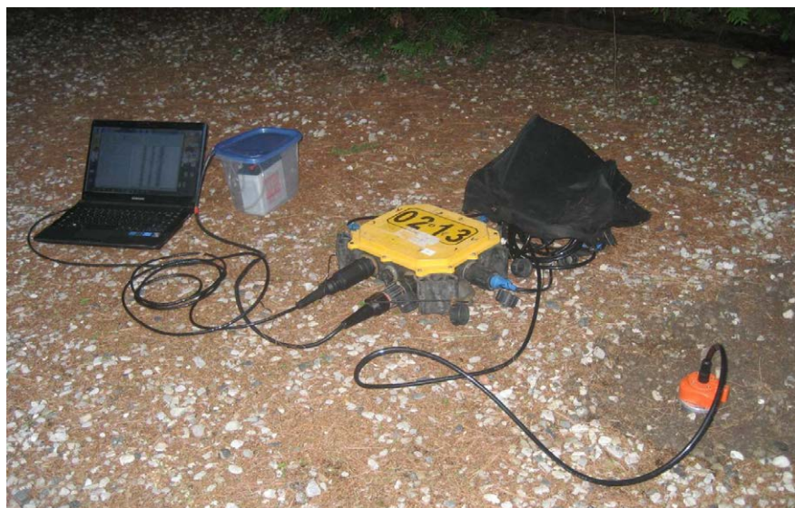
Figure 2. (R to L): Geophone, iSeis Sigma seismic recording node, 12V battery, laptop computer for downloading seismic data (courtesy Global Seismic Repairs, Calgary).
